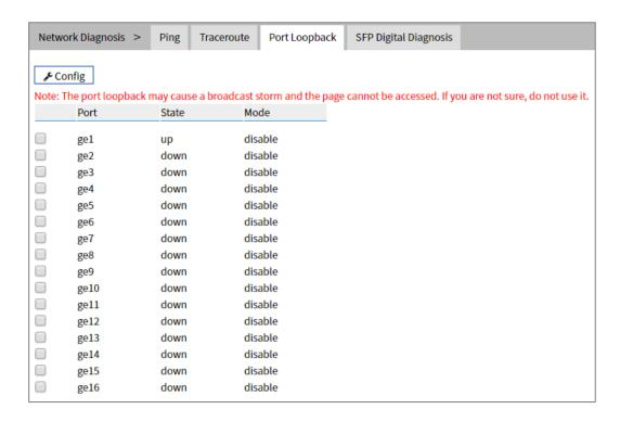
The main element configuration description of port loopback interface:
