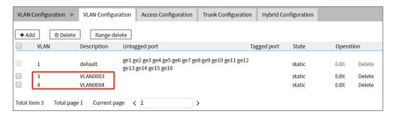
**Step 3** Set the corresponding pvid of port3 and port4, as well as the type of port2, port 3 and port4.
