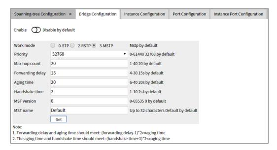
The main element configuration description of bridge configuration interface:
